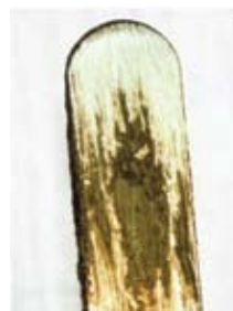
Figure 14 – Grooved Stainless Steel Blade Coated with Eschar
